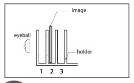
The first slit from the left is for simulating hyperopia (1) and the second slit is for simulating normal (2) and the third slit is for simulating myopia (3). (Please refer to the picture.) This simulation helps you study adjusting the strength of a lens of an ophthalmoscope. (Compartments for putting slides are provided on the holder. You can put 5 slides in each
