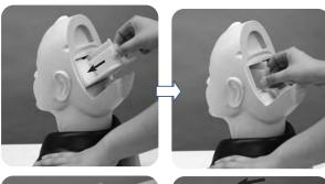
4. As shown in the picture, incline the slide holder a little and insert it into the eyeball unit.
